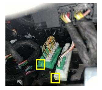
4. Plug the leads of the security module bypass into the CAN blocks.
